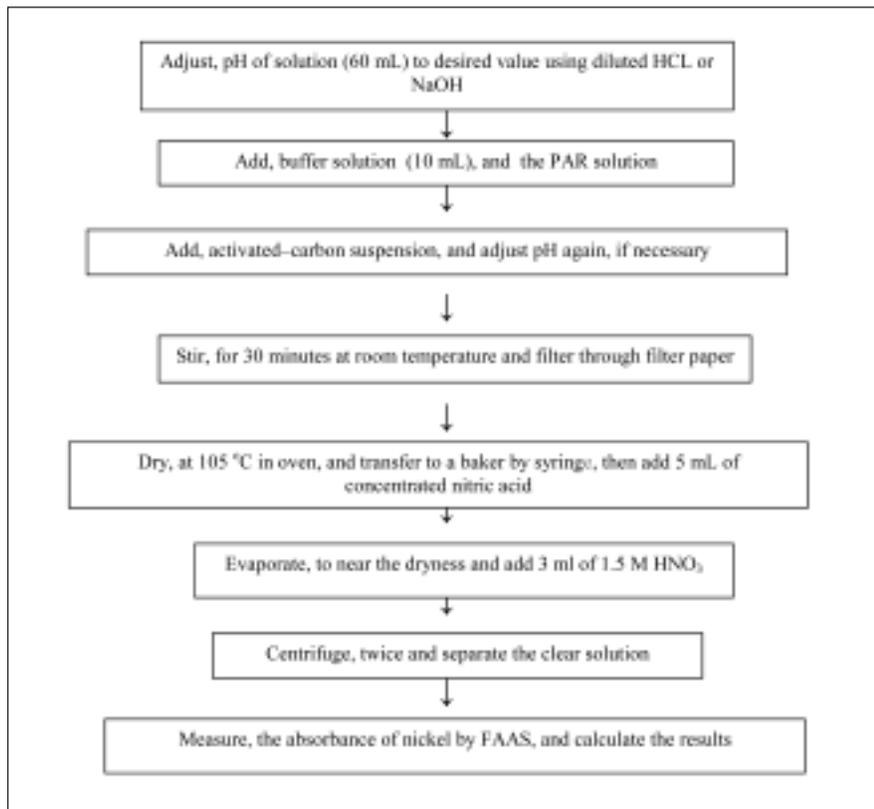
Fig. 1. Steps of analytical scheme in the enrichment procedure.
